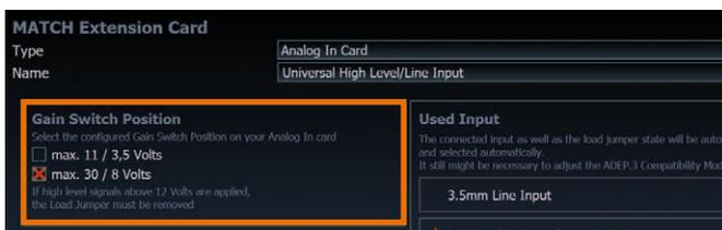
3. Adjust the input sensitivity to match the output voltage of the connected signal source.
