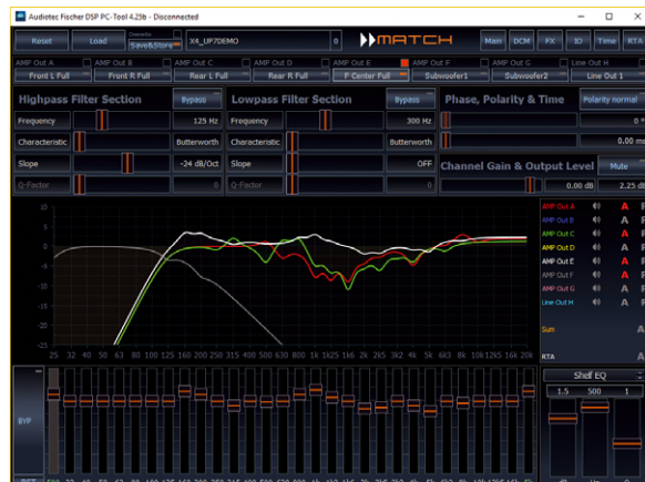
Settings for crossovers and equalizers are made in the main window. In addition, there is a mute button and dampers for phase and level
