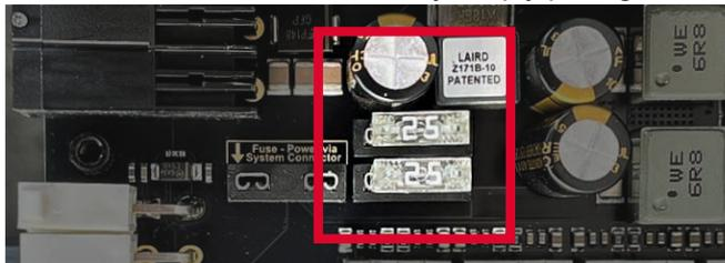
Then, insert one of the previously removed 25 A fuses into the “Fuse - Power via System-Connector” slot.
