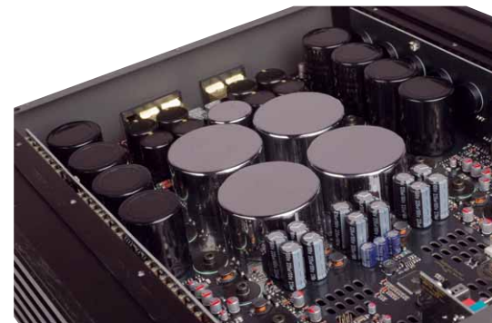
Specially produced buffer capacitors, hand-wound transformers and the storage chokes typical for Brax
