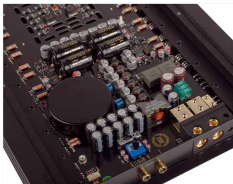
Voltage supply features a transformer core made from the vacuum melt
