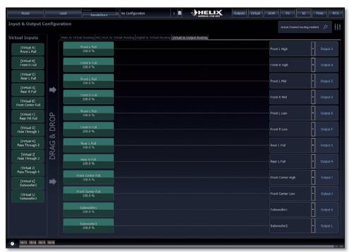
If VCP is activated, fi rst the inputs are routed to the virtual channels, then the virtual channels are routed to the outputs
