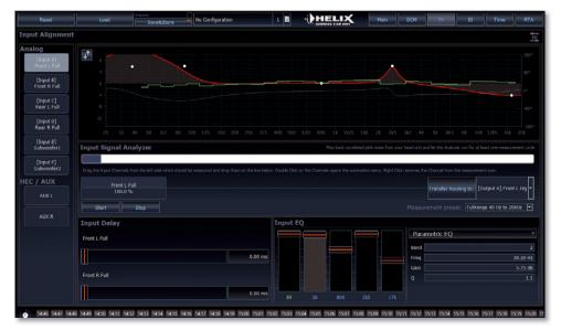
The ISA (Input Stage Analyzer) features single or combined measurment of the input channels. Time alignment and equalizing can be applied immediately
