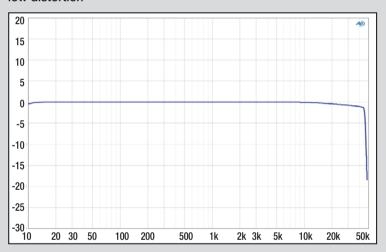
The P SIX DSP Ultimate shows an audio frequency range of up to more than 40 kHz thanks to the high sampling rate of the DSP and the high PWM frequency of the Class-D power amplifiers
