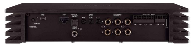
The 6 processed outputs are distributed over 4 RCA sockets and the digital optical output. The inputs feature 6 x RCA, 6 x high-in and digital, either optical or coax
