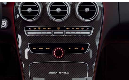
The LEDs change their color depending on the function, the colors can be perfectly adjusted to the vehicle lighting
