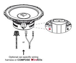
Option b: Universal connection via optional available CWK FX.W-550CC cable, e.g. in active applications
