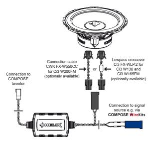
Ensure that all components are correctly connected in polarity, i.e. plus to plus and minus to minus. The positive leads of the loudspeaker system are marked red.
