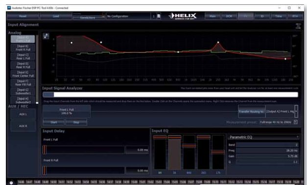
In the ISA, any inputs and their sums can be measured. EQ (with Allpass) and time alignment are adjusting the incoming signal.
