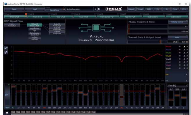
The setup of the virtual channels is similar to that of the output channels, only without crossovers. The virtual front EQ and FX front processing then affect all output channels routed from there.
