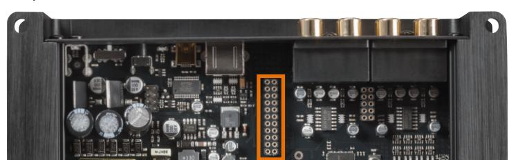
4. Make sure that the module is installed properly and all pins are fully inserted into the socket:
