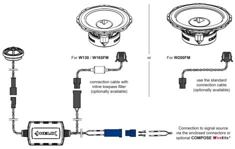
Ensure that all components are correctly connected (phase), i.e. plus to plus and minus to minus.
