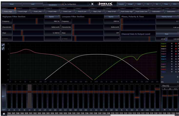
In the output menu you can set crossovers and equalizers for all output channels
