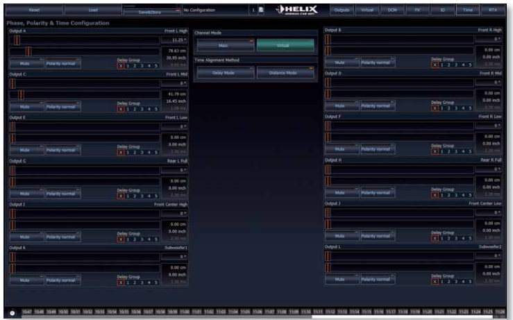
The time alignment is set either as distance or as time. As a special feature, the phase can be adjusted by a slider when a filter is set
