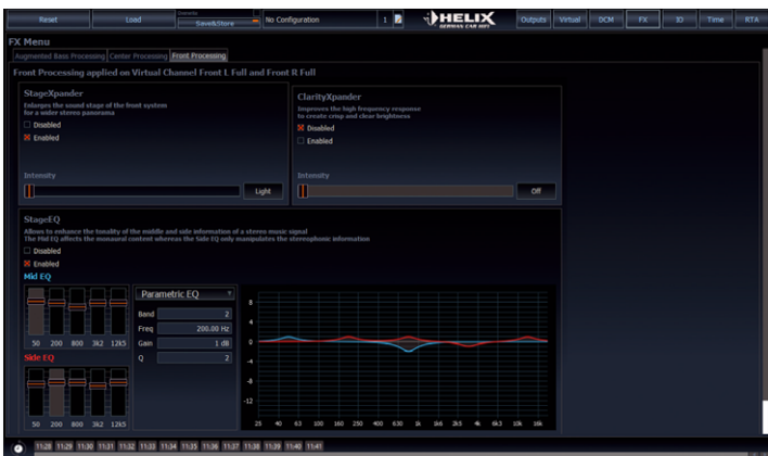
The front processing now includes a mid/side EQ, which can be used to control the stage centre and stage edges separately
