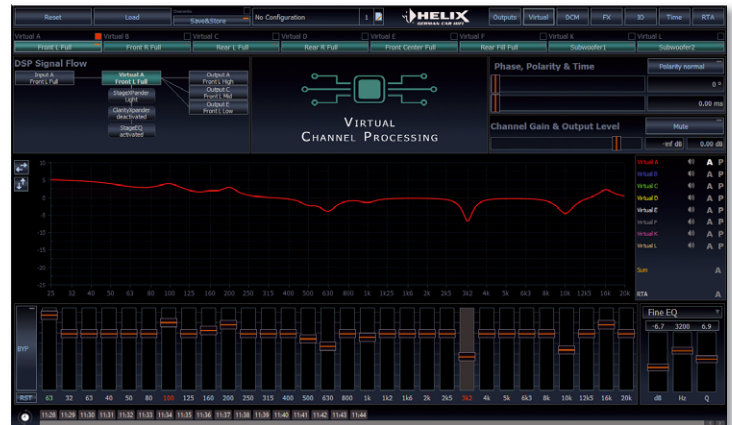
Routing Step 2: Now the 8 virtual channels are routed to the 12 outputs, e.g. a virtual front channel on tweeter, midrange, woofer and a virtual center channel on center woofer and center tweeter
